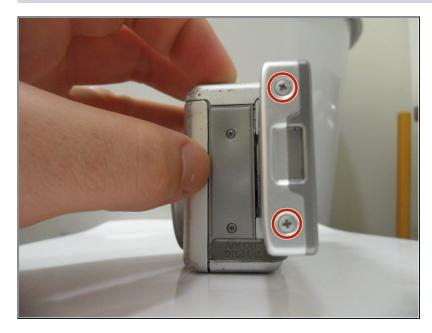
Using a Phillips #00 screwdriver, remove the two 2.9 mm screws on the side of the LCD screen.
