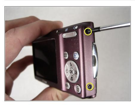
Unscrew the two 4.05mm screws on the side next to the buttons.
