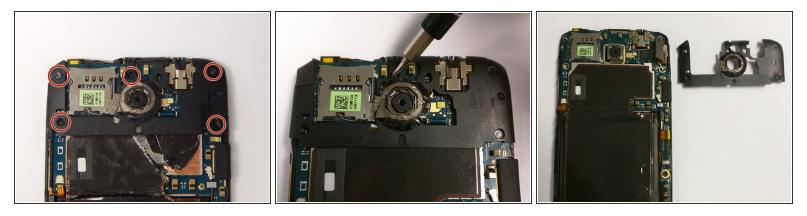
Remove the five 2.4mm screws using a Phillips head screw driver and then remove the plastic cover.
