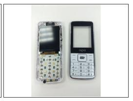
• Use the plastic opening tool to pry the front of the phone away from the back of the phone.
