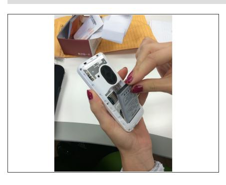
Remove the battery from the back of the phone.
