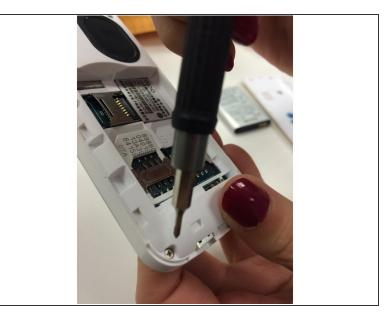
Unscrew the 5 screws on the back of the phone using the Philips Head 000 screwdriver.
