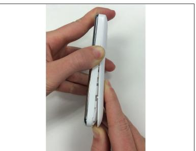
Insert thumb into the groove on the back lefthand corner of the phone to unsnap the back cover.
