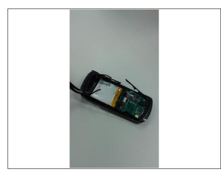
Use the tweezers to pry off the black and silver plastic that lines the edges of the device.
