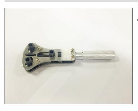
Next, you will have to adjust the dimensions of the watch back remover tool you will use to take the watch back off. The dimensions should be set so the tool properly fits the three connection points on the back of the watch. You can do this by screwing or unscrewing the adjustment screws on the tool.
