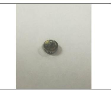
Use tweezers to carefully remove the current watch battery. Next, place the new battery in the same spot and orientation you removed the previous battery from.
