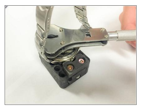
Place the back of the watch back on and align the watch back remover tool to the three connection points.
