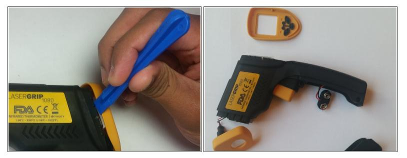
Using the plastic opening tool remove the front and rear yellow covers.
