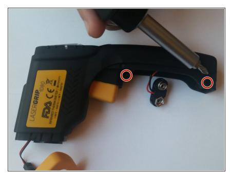
Remove the two 3.1 mm Phillips #0 screws.
