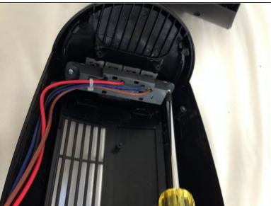
To get more maneuverability, remove the button panel. This can be done by removing the 2 screws on either side of the panel in order to fully remove it.
