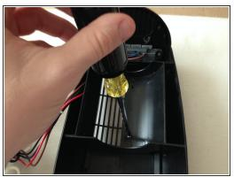
Once you have the fan apart, in order to get more maneuverability, the wire attached to the motor needs to be loosened. This can be done by removing the two screws highlighted in red.
