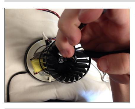
Tighten the bolt to the left and you have successfully installed your new fan blades.
