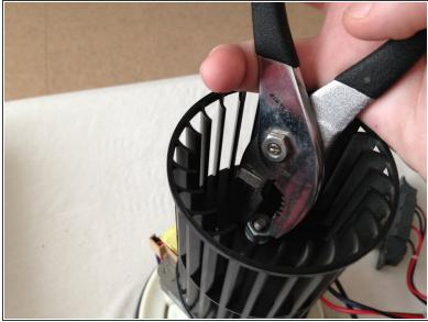
The bolt that you need to remove is inside of the pre-installed fan blades. With your pliers, grab a hold of the nut and twist to the RIGHT. This will allow you to remove the fan blades.
