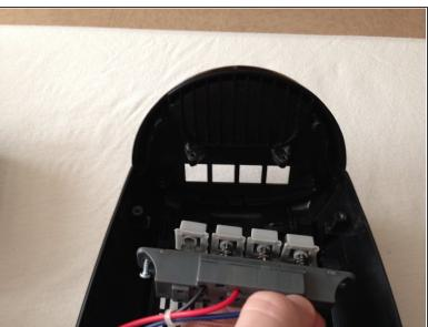
Carefully remove the panel by pulling on it. It should fall out easily and separate completely from its housing.
