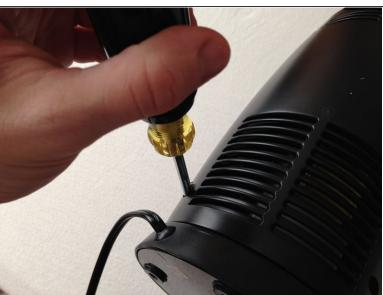
There are 6 screws holding the entire fan together, which need to be removed to access the internals of the fan.
