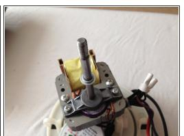
• In order to install the new blades, there are two pieces that you have to match up. The blades and pole both have a flat side that you have to match up in order for the blades to stay on.
