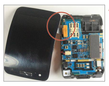
Locate the ribbon assembly attaching the display to the motherboard.
