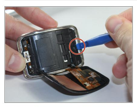
Use a plastic opening tool to gently pry upwards on the plastic motherboard assembly.
