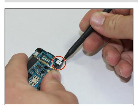
Use the spudger to lift up the white microphone circuit board.
