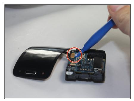
Use a plastic opening tool to detach the glass screen/ LED Display ribbon connector from the motherboard.
