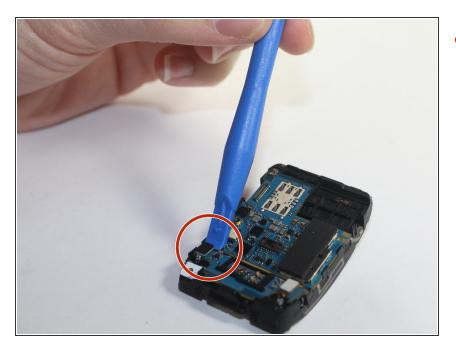
Use the plastic opening tool to lift up the microphone ribbon connector.
