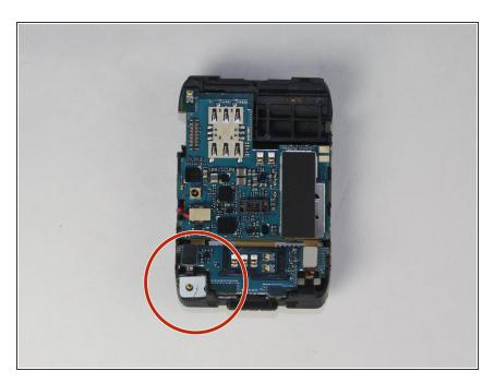
Locate the microphone on the lower right corner of the plastic motherboard assembly.
