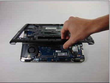
• Using the plastic opening tools, remove the plastic cover by beginning at one of the corners and prying it up.
