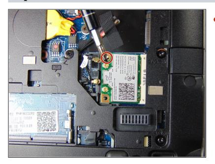
Phillips #1 screw securing the wireless card.
