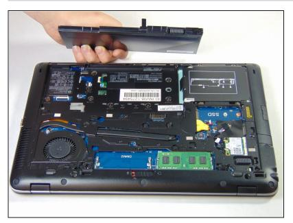
Battery should easily be lifted up and out.
