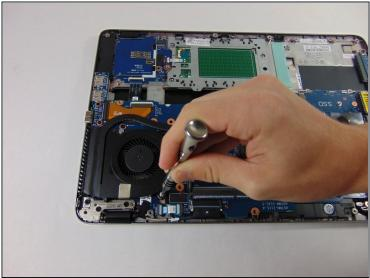
Loosen the six Phillips #1 screws. These will remain captive to the heatsink.
