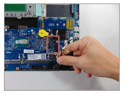
Disconnect the cables by taking off the tape and getting them out from under the plastic.
