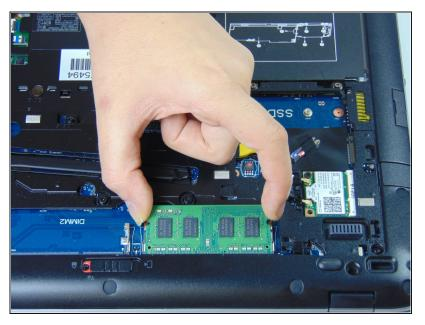
Pull the RAM stick gently out and up once the tabs have been pulled to the side.
