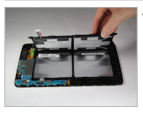
Now that all of the screws are removed and the cable is disconnected, lift the battery upwards to remove it from the device.
