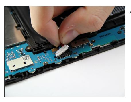
Disconnect the battery cable from the motherboard by grabbing the cable and pulling upwards.
