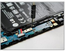
Remove the twelve 4 mm Phillips #000 screws surrounding the perimeter of the battery.
