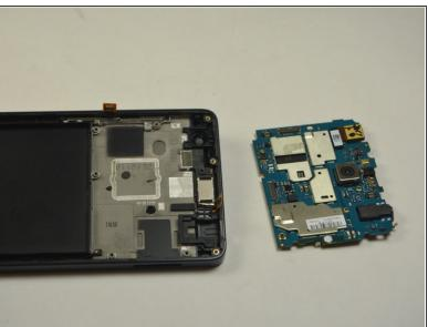
Wedge the plastic opening tool, between the motherboard and the inner region of the phone in the slot atop the motherboard.
