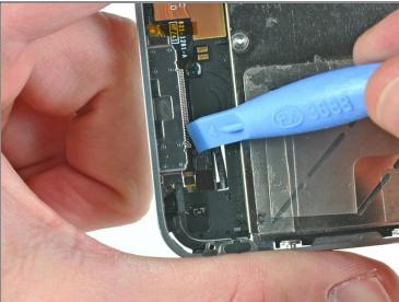
• Use a clean fingernail or the edge of a plastic opening tool to flip up the retaining flap on the home button ribbon cable.
