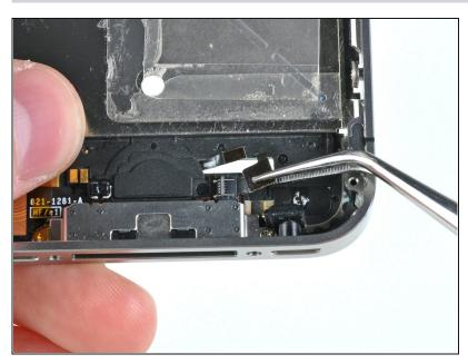
Use a pair of tweezers to pull the home button cable out of its socket.
