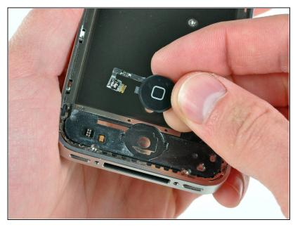
Carefully de-route the home button cable through its slot in the outer case and remove it from the iPhone.
