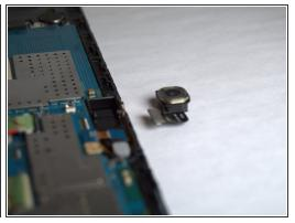
Use a spudger to disconnect the camera from the motherboard and then remove the camera.
