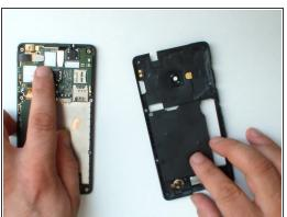
• With a plastic opening tool separate the back cover from the middle frame.
