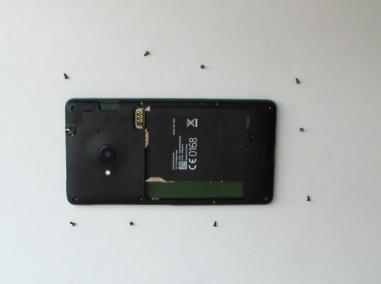
With a screwdriver Torx T4 remove the 9x screws.
