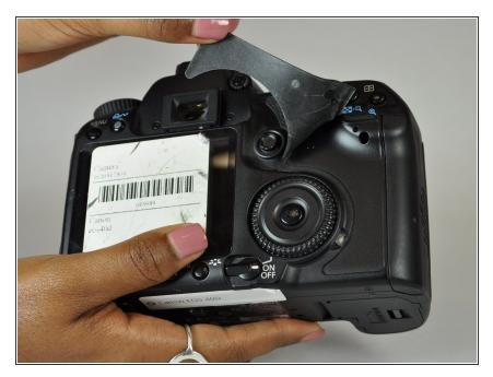
Peel off the grip material from the body of the camera, exposing the screws.
