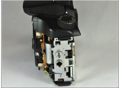
Remove the side panel by unscrewing three 5 mm JIS #000 screws.
