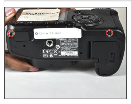
Remove the two 3.0 mm Phillips #000 screws on the bottom of the camera.
