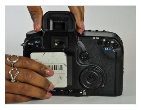
Remove the rubber eyepiece by sliding it upwards.
