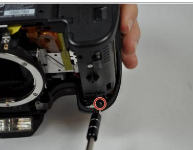
Remove the two 5 mm screws from under the wheel and under the shutter button using a JIS #000 screwdriver.
