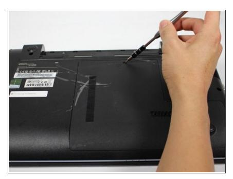
Remove this 4 mm Phillips #8 screw using a Phillips #00 screwdriver.
