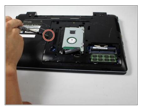
Remove the 4 mm Phillips #8 screw to the left of the hard drive using a Phillips #00 screwdriver.
