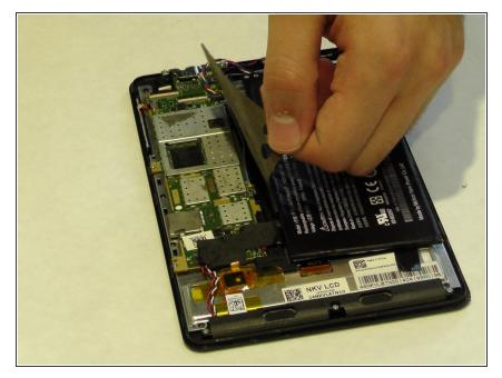
• Carefully peel back the copper foil to reveal the motherboard.
