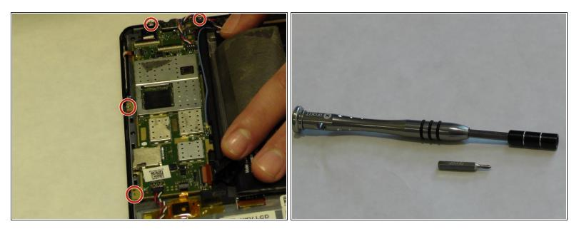
Use a JIS screw bit #00 to remove screws around the motherboard using the provided image to locate each screw.
