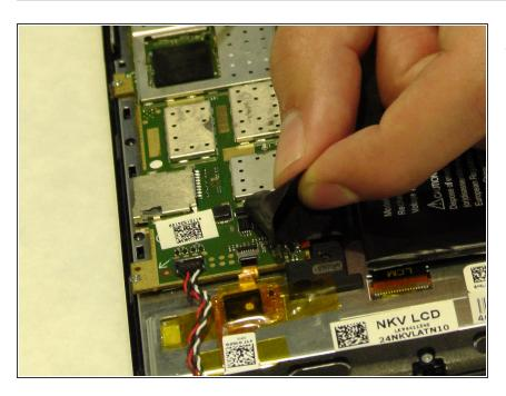
• Peel tape back to expose connections.
