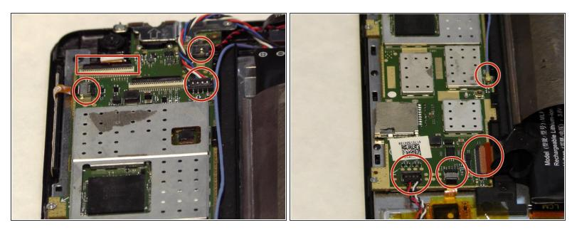
• There are several sets of wires connected to the motherboard as shown in the images. Carefully disconnect each set of wires.
