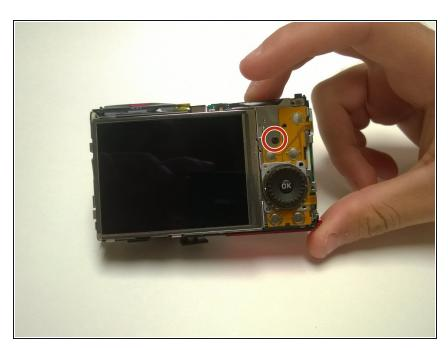
Using a Phillips #00 screwdriver, remove the PH 2mm screw located to the right of the screen, above the OK dial.
