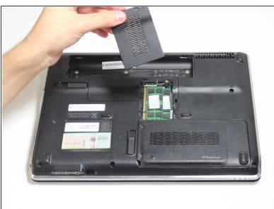
Lift the RAM case cover after the screw has been loosened.
