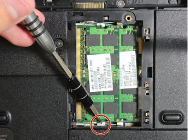
Locate the 2 silver release buttons inside the RAM socket, indicated in the pictures. They are on opposite sides of the socket.
