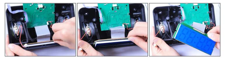
• Remove the screen by pushing it toward the middle of the clock and pulling it up out of the clock.
