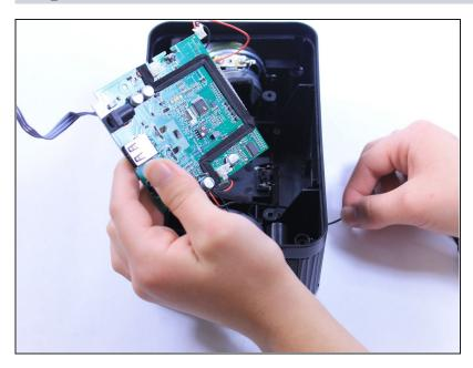
• Pull the radio antenna the rest of the way through the side of the clock.
