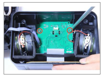
• Unscrew the two 10mm screws from the bottom circuit board.
