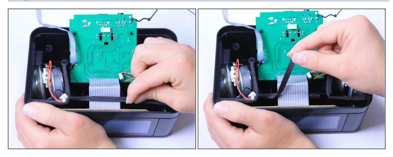
• Lift the adhesive strip that holds down the grey ribbon cable which attaches to the circuit board and the LCD screen.
