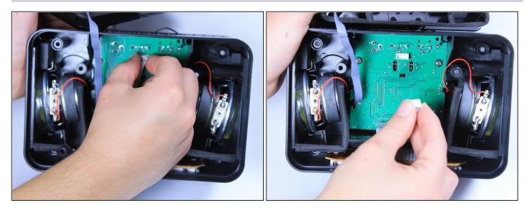
• Grip the white ribbon cable connector that attaches the lightning cable to the middle of the central circuit board located in the bottom of the clock. Pinch and pull straight up to detach the cable.
