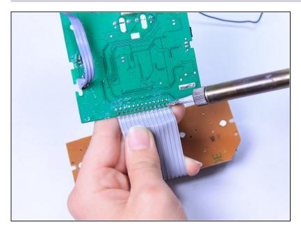
• Use this <u>soldering guide</u> to remove and replace the cable and screen.
