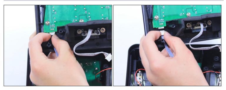
• Remove the white ribbon connector that connects the central circuit board to the circuit board attached to the top of the clock by gripping it on both sides and pulling it straight away from the board.
