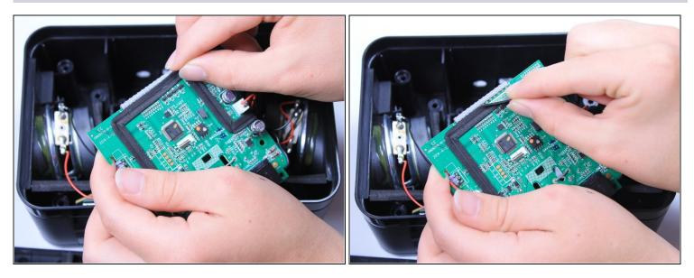
• Lift the adhesive strip that covers the connections between the grey ribbon cable and the circuit board by peeling it off of the circuit board.
