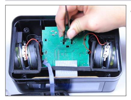
Once the ports on the back of the circuit board are displaced and resting against the back of the clock, use a pair of <u>tweezers</u> to lift the circuit board up off of the bottom of the clock, continuing to feed the radio antenna through the side of the clock as the board lifts up.
