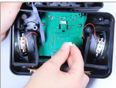
Grip the white ribbon cable connector that attaches the lightning cable to the middle of the central circuit board located in the bottom of the clock. Pinch and pull straight up to detach the cable.
