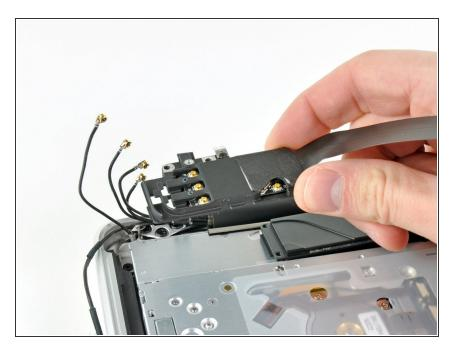
Remove the AirPort/Bluetooth assembly, minding the fragile antenna contact near the corner of the upper case.
