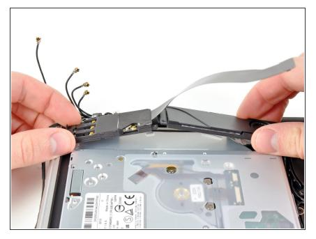
Pull the AirPort/Bluetooth assembly and the Subwoofer upward near the center of the side of the optical drive until they clear each other.
