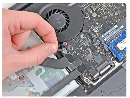
• Carefully pull the camera cable out of its socket on the logic board.
