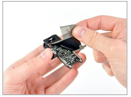
Continue peeling the EMI tape off the bottom of the AirPort/Bluetooth bracket and remove it from the assembly.
