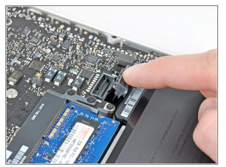
Bend the battery cable slightly away from its socket on the logic board so it does not accidentally connect itself while you work.
