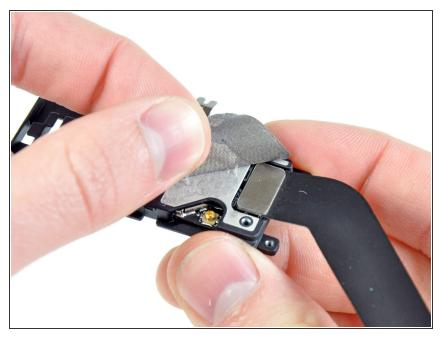
Peel back the piece of EMI tape covering the AirPort/Bluetooth cable connector.
