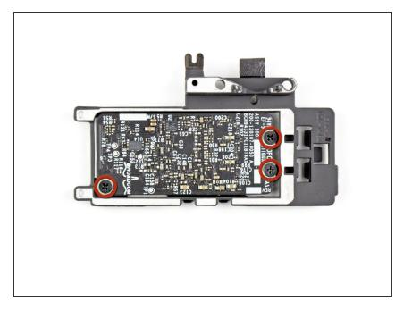
Remove the three 3 mm Phillips screws securing the AirPort/Bluetooth board to its bracket.
