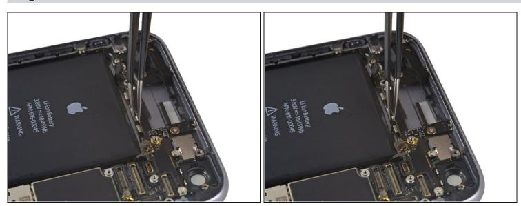
• Deroute the upper left cellular antenna cable from the first logic board clip by nudging it out from under the clip, towards the battery.
