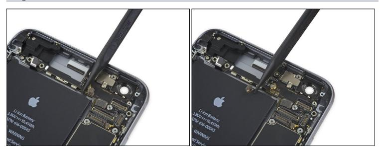
• Disconnect the cellular antenna cable by prying its connector straight up from its respective socket on the logic board.
