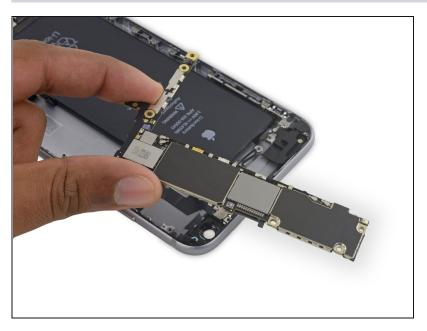
• Remove the logic board.
