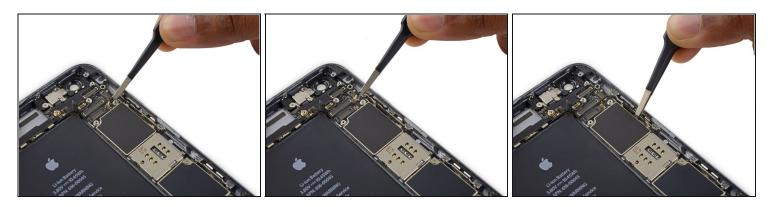
• Deroute the antenna cable from the two clips on the right edge of the logic board.
