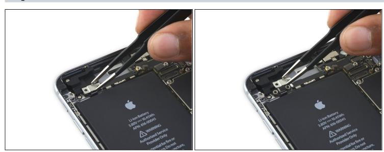
• Remove the audio control cable bracket.
