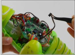
• Use tweezers to remove all of the colored wire connectors from their sockets on the circuit board.
