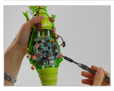
Remove the three 7.2 mm Phillips #0 screws connecting the main circuit board to the body of Zoomer Dino Boomer.
