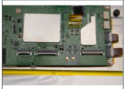
• Disconnect the two plastic connectors overlapping the battery from the motherboard.
