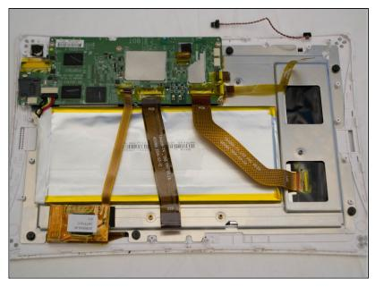
i Before removing the battery, be aware that it is held together by a strong adhesive. The battery itself is very malleable and flimsy, so make sure to handle it with care.
