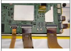
• Remove the remaining yellow plastic film from the surrounding connectors so that the battery can be easily removed.
