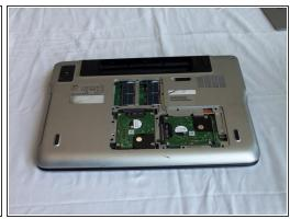
Lift the module cover by inserting a plastic opening tool into the crevice near the screw and lift upwards.
