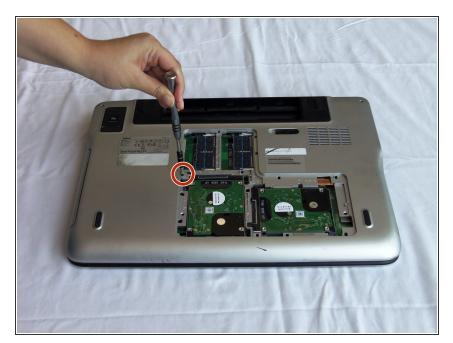
Unscrew the screw holding the optical drive with a Phillips screwdriver.
