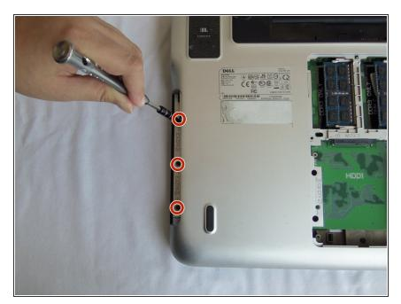
Unscrew three 4mm screws near the edge of the optical drive compartment with a Phillips screwdriver.
