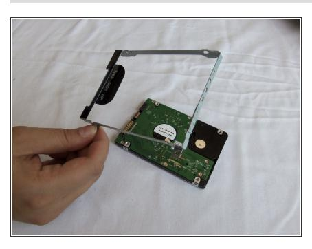
Remove the hard drive casing.
