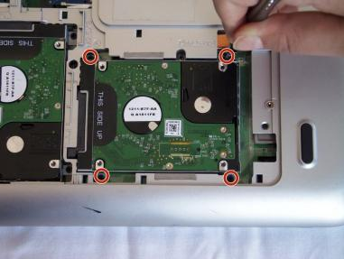
• Remove the four 4mm Phillips screws fastening the first hard drive.
