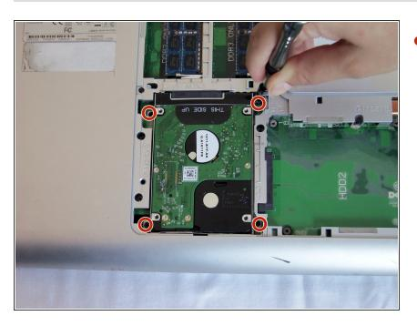
Remove the four 4mm Phillips screws on the second hard drive.
