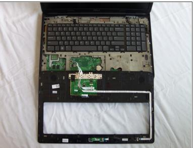
Gently lift and rotate the palm rest panel until it's upside down as it is still connected by the mouse pad wires.
