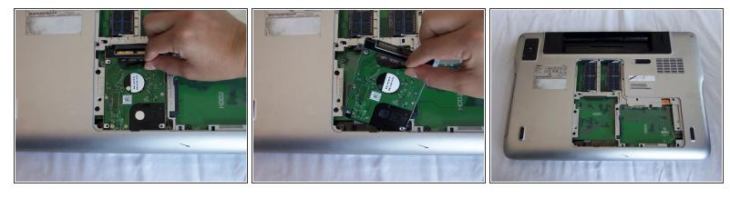
Using the tab that says "THIS SIDE UP," pull away from the laptop to remove the hard drive.
