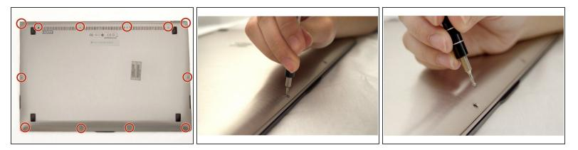
Remove the twelve 3 mm bottom panel screws with a <u>T5 Torx Screwdriver</u>.
