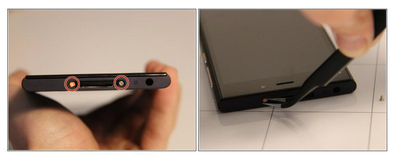
Remove the two Phillips head screws located at the top of the phone on either side where the SIM card was ejected.
