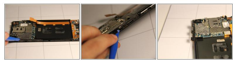
Using a pry tool, gently lift the side control buttons assembly away from the case. They should be loosely connected to the motherboard.
