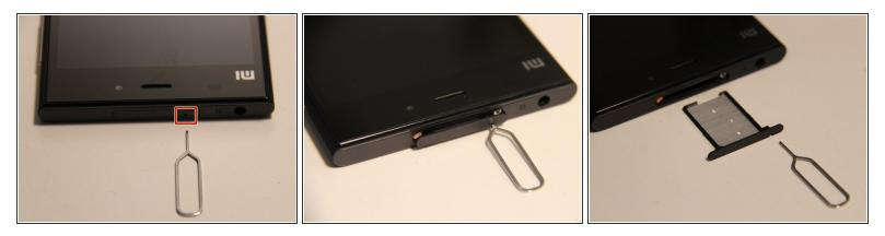
• Firmly press the SIM card removal tool into the hole located at the top of the phone to eject the SIM card tray from the slot.
