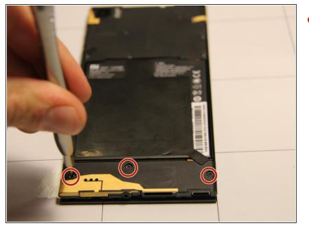
Next, remove these three screws located at the bottom of the back panel.
