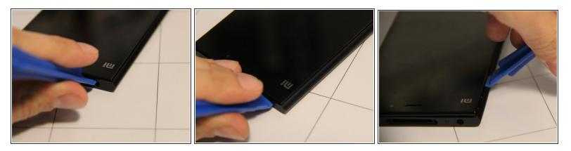
• Insert a pry tool into the upper edge of the phone, where there is a small gap between screen and frame of the phone to begin separating the screen from the rest of the phone.
