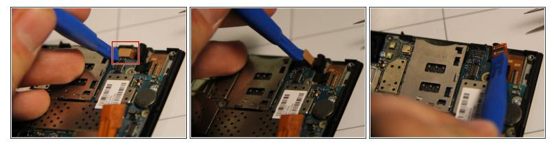
Separate a cable ribbon from the top right of the motherboard - near the cable from the previous step - by gently inserting the pry tool under the rectangular metallic piece and lifting.
