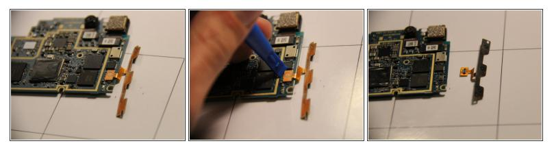
• With the motherboard removed flip it over onto its front and use a small pry tool to gently disconnect the side buttons from the back of the motherboard.
