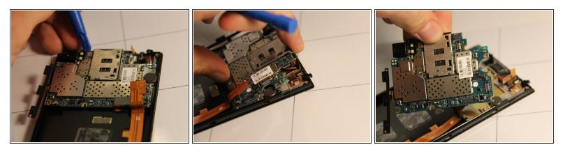
• Remove the motherboard from the panel carefully. Use the pry tool as a lever from the top of the panel and lift if from that side.
