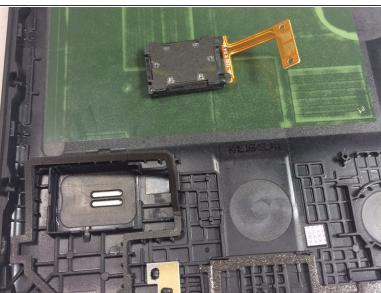
Now you should be able to lift the speaker out of it's small fitting with the tweezers.
