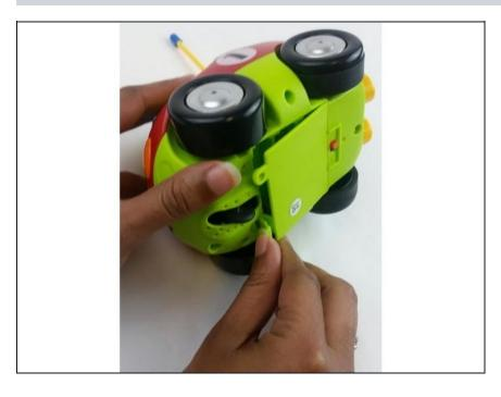
Pull up the tab to reveal the battery compartment.
