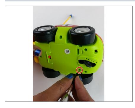
On the bottom of the car, unscrew the 6.2 mm screw that houses the batteries using a Philips 00 precision screwdriver.
