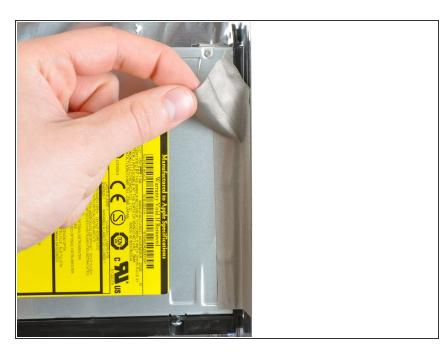
Peel off the strip of EMI tape attaching the right side of the optical drive to the rear case.
