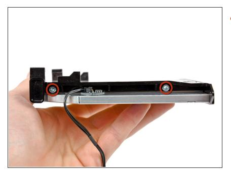
• Remove the two T10 Torx screws from the side of your optical drive.
