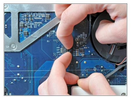
Pull the optical drive thermal sensor connector toward the right side of the iMac to disconnect it from the logic board.
