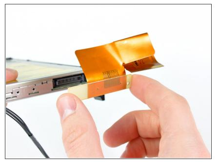
• Pull the optical drive cable connector away from the optical drive.
