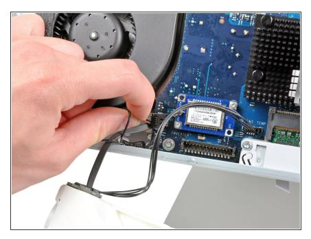
Pull the CPU fan cable toward the left side of the iMac to disconnect it from the logic board.
