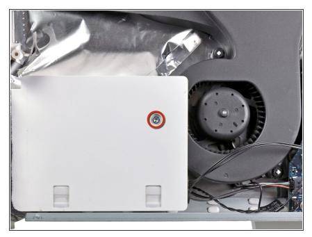
Remove the single 38 mm T10 Torx screw securing the left speaker to the rear case.
