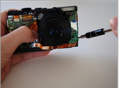
On the front motherboard, unscrew the one bottom right 3 mm Phillips head screw.
