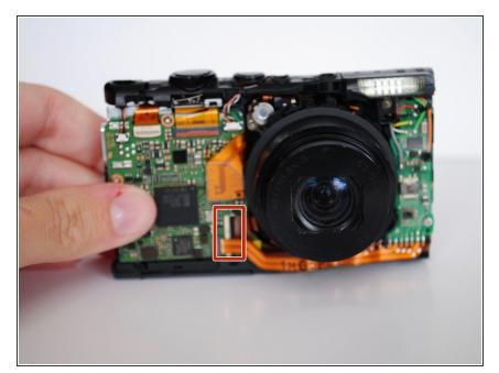
Using a plastic spudger, remove the bottom front ZIF connector.
