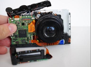
Using your hands, carefully lift the flash housing up and remove it from the area.
