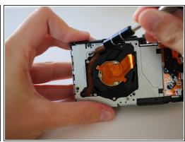
Unscrew the four 3 mm Phillips head screws attached to the metal casing on the back of the camera, behind where the LCD screen once was.
