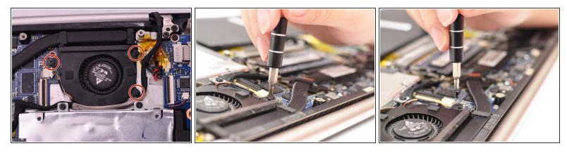
Remove the 3 (4mm) fan screws with a <u>Phillips #0 Screwdriver</u>
