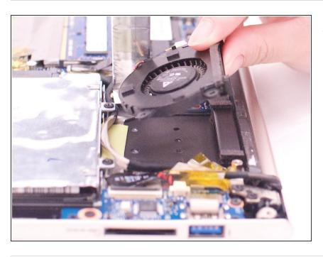
Remove the fan completely.
