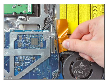
Pull the optical drive ribbon cable out of its socket, being careful not to rip it in the process.
