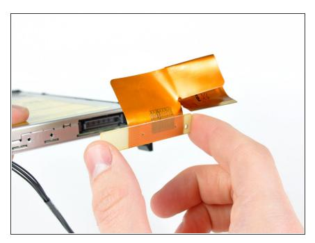
Pull the optical drive cable connector away from the optical drive.
