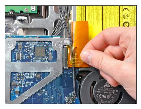
Remove the strip of tape covering the optical drive cable connector.
