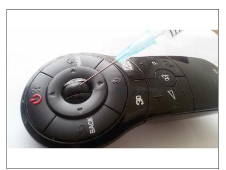
Press the injection needle into the rubber wheel until you feel the ridged axle
