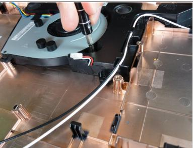
Remove the two screws shown with the Philips #1 screwdriver.
