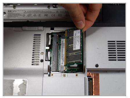
Gently lift the the RAM up and out of its seat.
