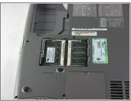
Remove the single screw securing the RAM compartment and pull up to reveal the RAM.
