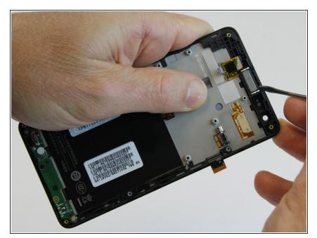
Using the nylon or metal spudger, gently pry the front speaker from the screen assembly.
