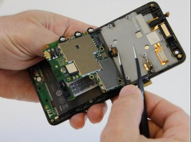
Using one prong of the tweezers, lift and pry back the metal clip positioned over the front proximity sensor ribbon connector.
