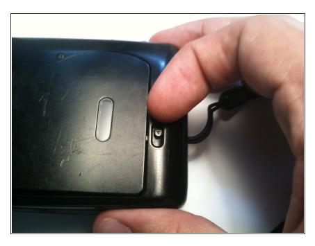
Open the back door on the camera by pushing down on the door latch.
