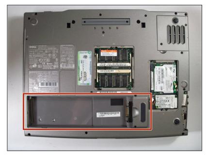
• Remove the battery from the bottom left of the laptop as shown.
