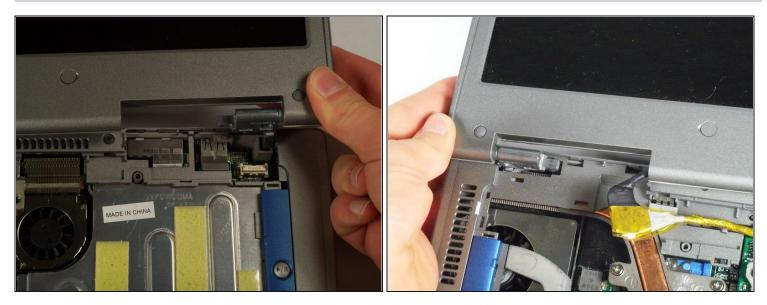
• Lift the display module directly upwards from the base of the computer.
