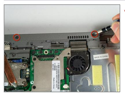
Remove the two screws holding down the upper case with a Phillips #1 screwdriver.
