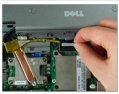
Disconnect the video card from the display module by gently lifting upwards on the black tab.
