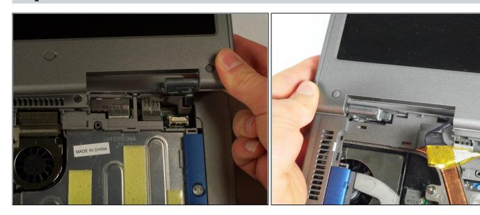
• Lift the display module directly upwards from the base of the computer.
