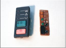
• Use a metal spudger to remove the control panel and its circuit board from the top cover.
