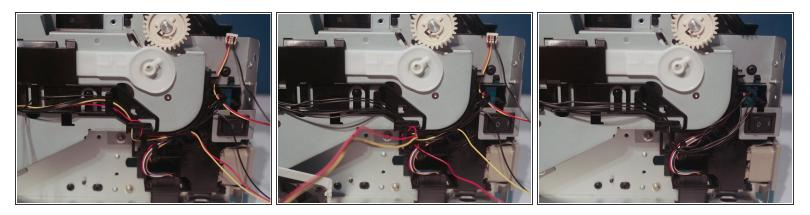
• Remove the fan cable from the cable guide.
