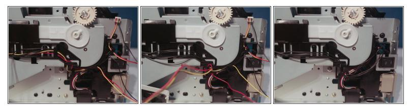
• Remove the fan cable from the cable guide.
