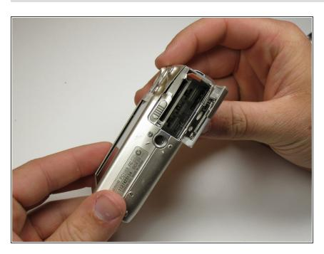
Remove the battery and SD card from the camera.
