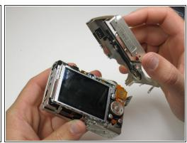
Gently lift the rear of the case to remove it from the camera.
