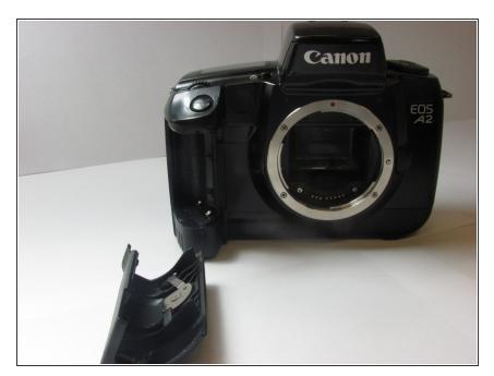
Remove the battery from inside the battery housing and set the cover aside.
