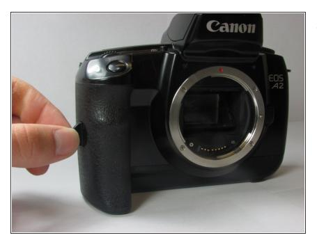
Locate the battery door/camera grip on the left side of the camera and lift the rotating removal tab.
