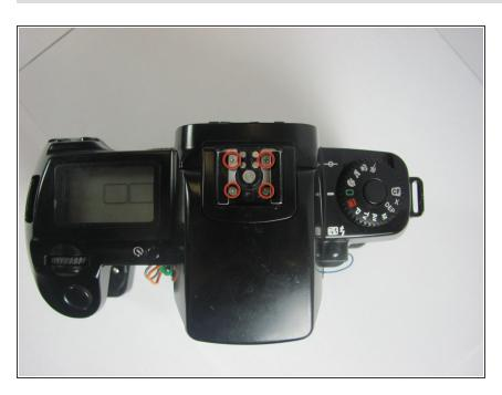
Loosen, but do not remove, the 4 screws on top of the flash shoe.
