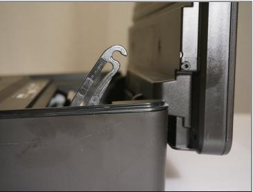
• Gently pull on the hook. Retain the scanner glass and the cover once the hook is removed.
